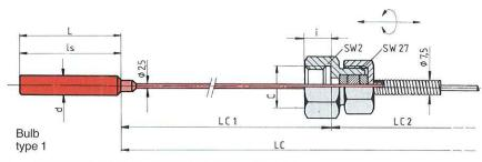
$L_C$  = Total length of capillary between thermometer head and bulb.
