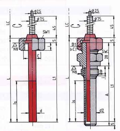
Fixing by cap connection (sealed)
