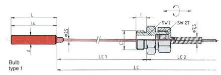
L<sub>C</sub> = Total length of capillary between thermometer head and bulb.
