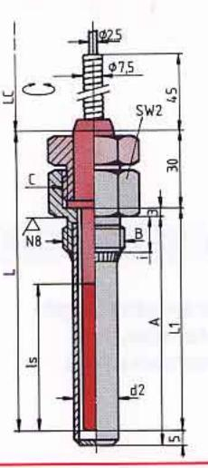
Fixing by swivelling threaded connection (sealed)
